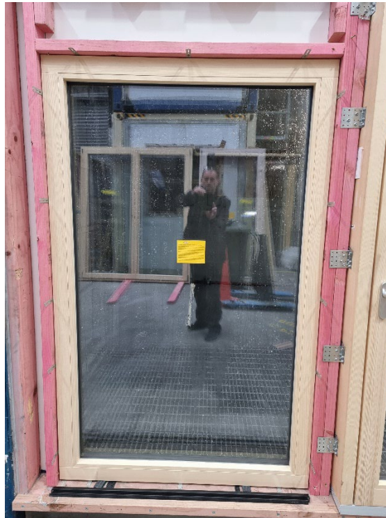
Photo 1: Interior of the Neuffer fixed light window installed in the test booth.
