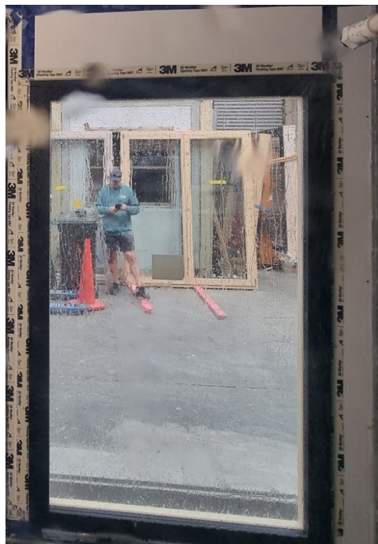
Photo 2: Exterior of the Neuffer fixed light window installed in the test booth.
